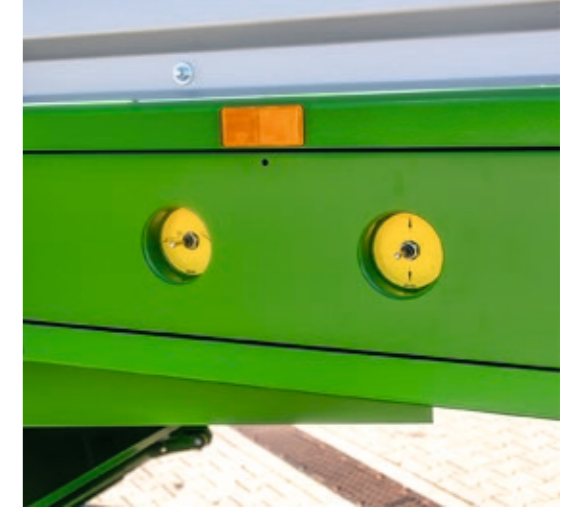
The drawbar and knife beam can be easily adjusted on the left side of the vehicle.
