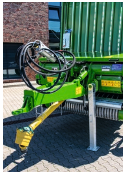
REPEX models 29 S / 30 K / 31 S / 32 K are equipped as standard with high drawbar and 40 mm towing eye. The low drawbar is optionally available.
