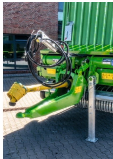
On the REPEX models 32 S / 33 K / 34 S / 35 K the low drawbar and K 80 ball hitch are standard.
