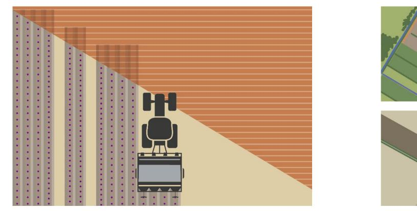
With the headland function, surfaces can be disabled for processing to work the field interior first, e.g. for planting potatoes as well as plant protection.
