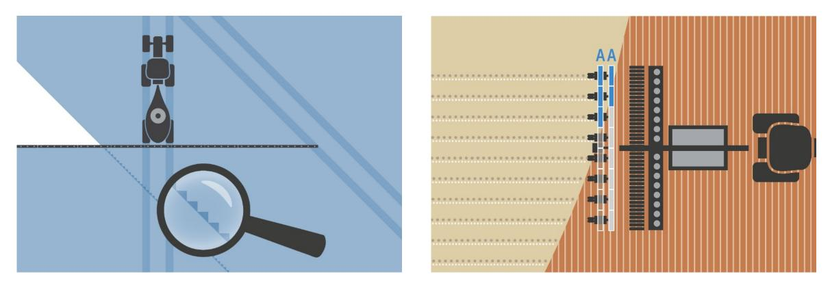
Section Control automatically switches up to 254 sections from one machine and up to four independent Booms.
