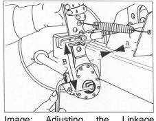
Image: Adjusting the Linkage Control Element
