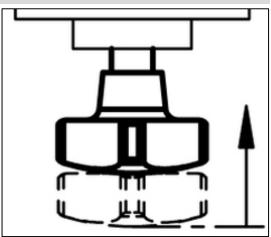
With such a system, the hand wheel must be turned in to the stop.
