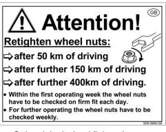
After initial operation of a new vehicle and after a tire change the wheel nuts must be retightened after driving 50 km. Furthermore, the nuts must be retightened after 150 km of driving and again after 400 km of driving.
