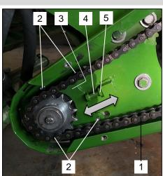
Image 58: Tensioning plate with tensioning bolt
