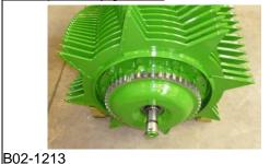
Filling quantity 2.7 Litre Gearbox oil: ISO VG 460 Syntheticoil
