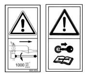
Only couple the PTO shaft when the motor is off, the PTO shaft is disengaged and the ignition key has been removed!
