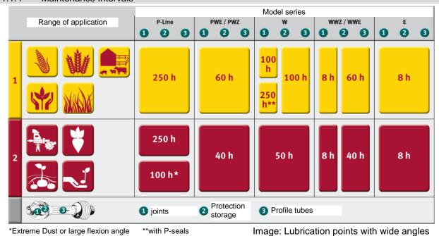
Application-specific maintenance provides for a reduction in maintenance costs. It was for this purpose that GKN Walterscheid introduced maintenance classes. What maintenance is now required for GKN Walterscheid shafts is easily seen on an application-specific maintenance chart. (The new maintenance intervals were confirmed by GKN Walterscheid through an intensive, five-year testing program.)
