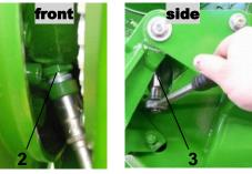
Image: Removing drain plug
