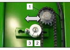
Image 61: Chain tensioning block
