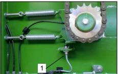
Fig. 1: Dosing Unit Sensor Left
