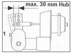
Image: Brake cylinder stroke
