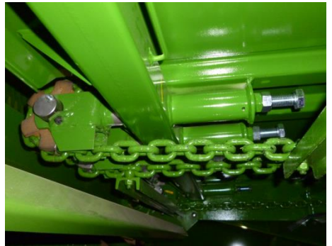
Image: Tensioning system
