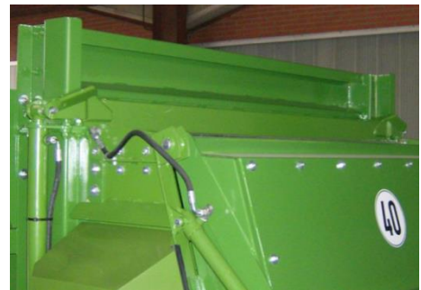
Image: Dosing wall extension
