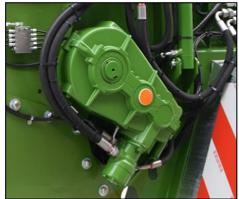
Image 18: Scraper floor drive
