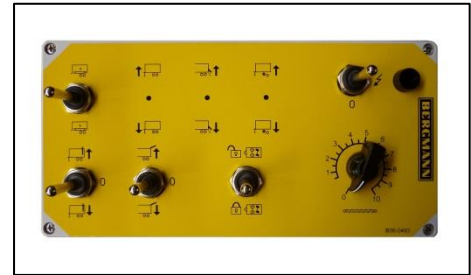
Image 65: Pilotbox Spreader terminal
