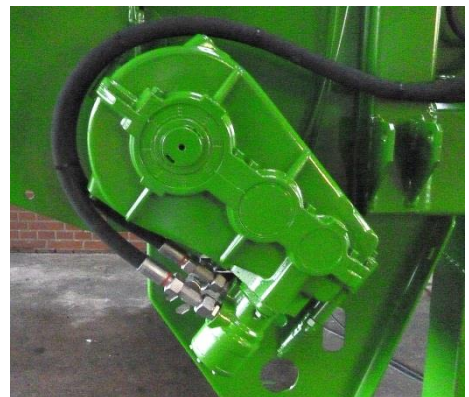
Image: Scraper Floor Drive
