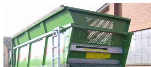
Image: Extension Walls 450mm (inclined)
