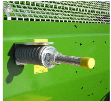
Image: Tensioning system
