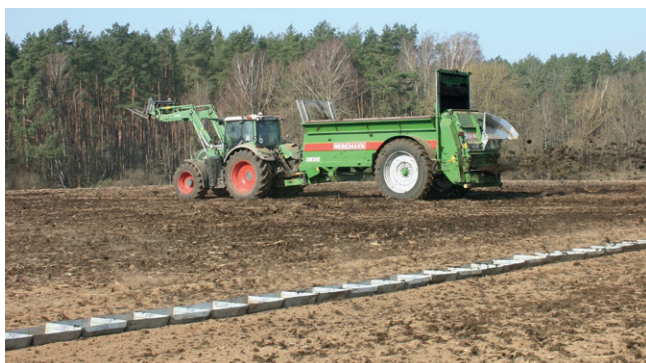
Fig. 2: The mobile test stand for measuring the distribution across rows
