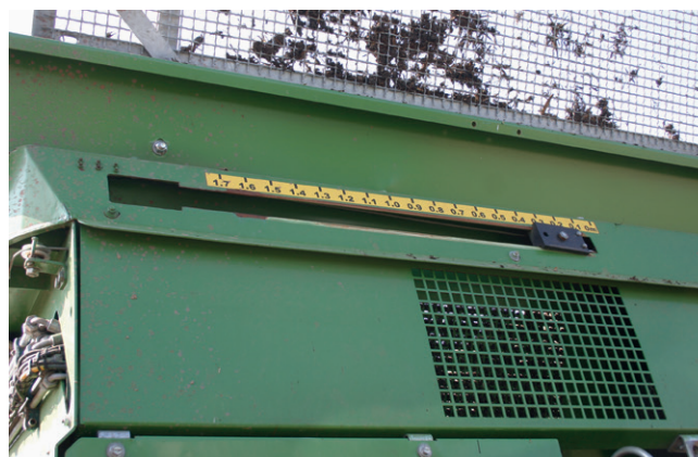
Fig. 5: This scale on the headboard indicates the current aperture of the slurry gate upstream of the beaters
