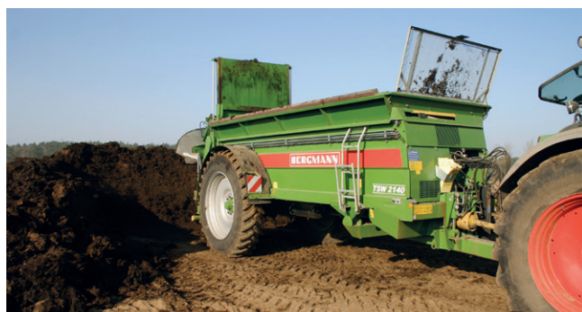
Fig. 3: BERGMANN TSW 2140 E with V-Spread is unloading the material during the measurements on application along rows
