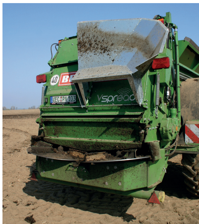
Fig. 6: The V-Spread discs in chevron-style arrangement
