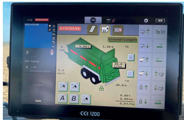
Fig. 4: The CCI 1200 terminal for BERGMANN TSW2140E with V-Spread
