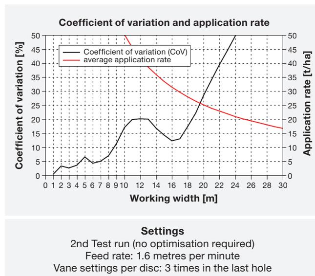
Fig. 10: Coefficient of variation relative to the work width when applying manure at 30 t/ha
