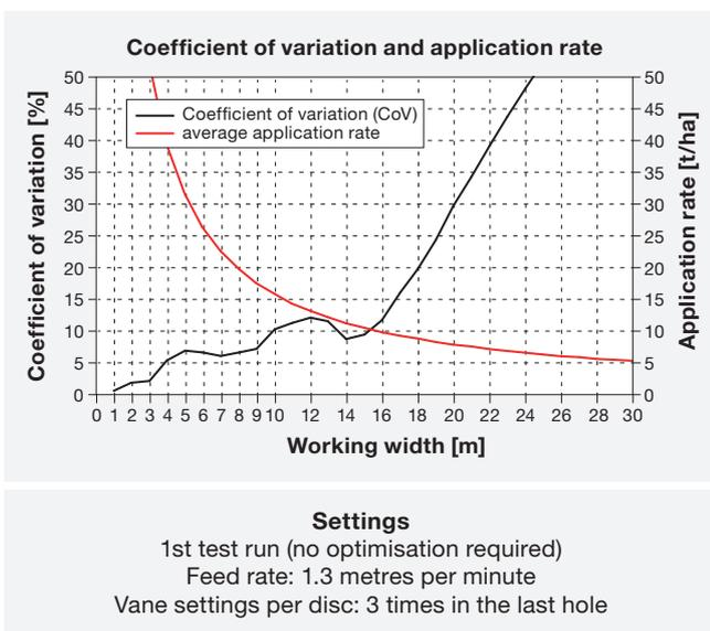
Fig. 8: Coefficient of variation relative to the work width when applying manure at 10 t/ha
