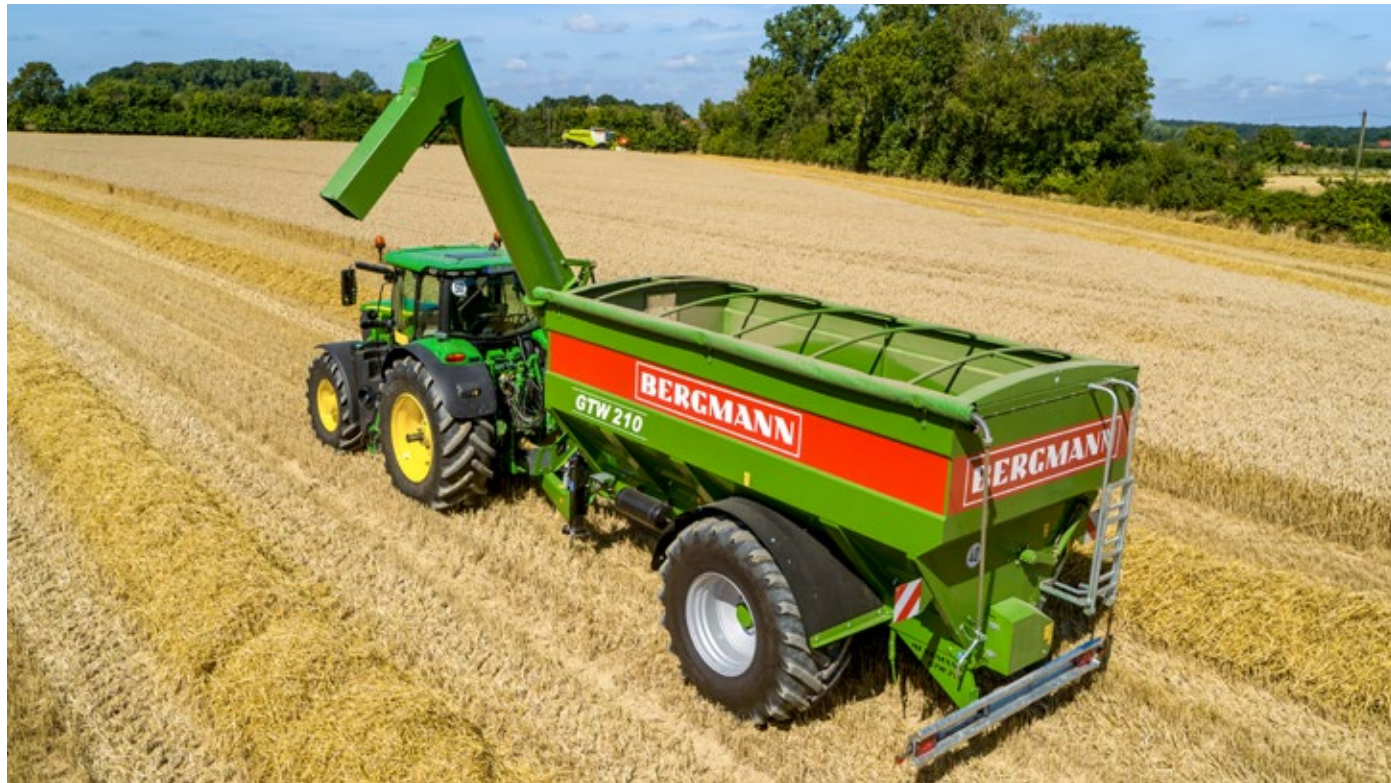
GTW 210 With a load volume of 21 m 3 , the GTW 210 is the entry-level transfer trailer from BERGMANN. The transfer rate is approx. 400 t/h.
