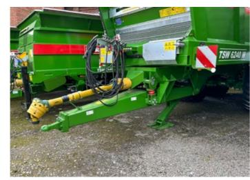
Various drawbar eyes are available for coupling. The standard ball coupling offers superior driving comfort at minimum wear. The hydraulic hoses are stored neatly in the hose cabinet, where they are protected from soiling.
