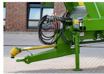
Various drawbar eyes are available for coupling. The optional ball coupling offers superior driving comfort at low wear. The hydraulic hoses are stored neatly in the hose cabinet, where they are protected from soiling.
