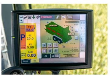
Also optionally available are additional AUX-N control devices, such as the CCI A3 multi-function lever and a connection to the TC Task-Controller (operating status, documentation, selective spreading (VRC), Section Control (SC), etc.). On the tractor, only a single-acting control unit and an unpressurised return are required. Load sensing is optionally available.
