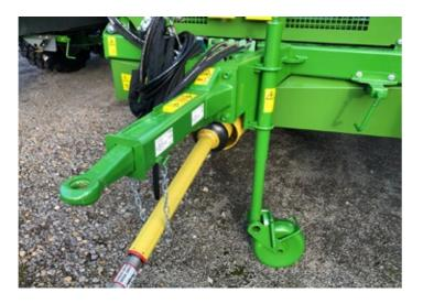
The drawbar eye is always a standard type eye with 40 mm diameter. The hydraulic hoses are stored neatly in the hose cabinet, where they are protected from soiling.
