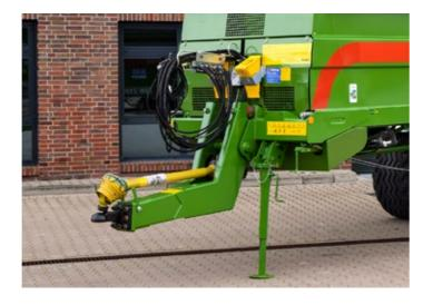
Various drawbar eyes are available for coupling. The optional ball coupling offers superior driving comfort at minimum wear. The hydraulic hoses are stored neatly in the hose cabinet, where they are protected from soiling.
