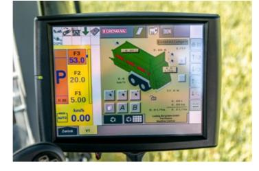
Also optionally available are additional AUX-N control devices, such as the CCI A3 multi-function lever and a connection to the TC Task-Controller (operating status, documentation, selective spreading (VRC), Section Control (SC), etc.). On the tractor, only a single-acting control unit and an unpressurised return are required. Load sensing is optionally available.
