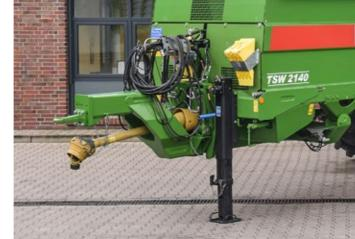
Various drawbar eyes are available for coupling. The standard ball coupling offers superior driving comfort at minimum wear. The hydraulic hoses are stored neatly in the hose cabinet, where they are protected from soiling.
